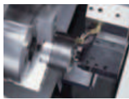
Turn outer diameter and facing (rough)
