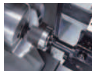
Turn outer diameter and facing (finish)
