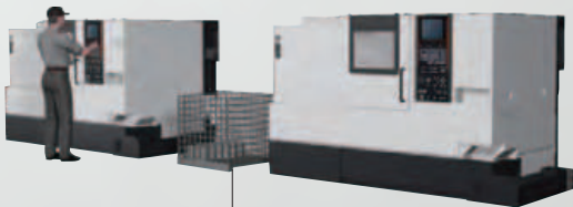
In-process inventory between processes
