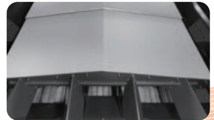
Enlarged chip ducts for smooth chip disposal
