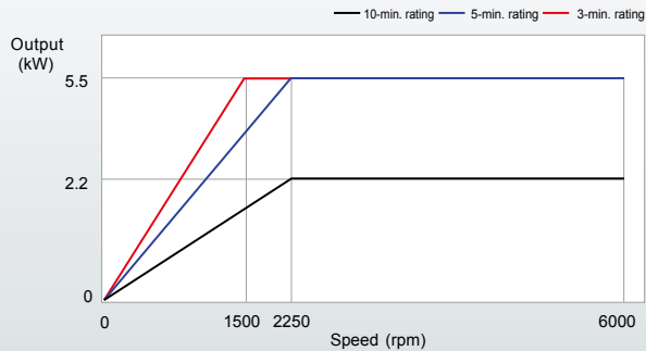
Rotary tool spindle output/torque diagram
