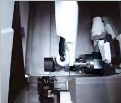
Unloading finished workpiece
