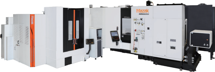
PALLETECH MANUFACTURING CELL (1 level)
