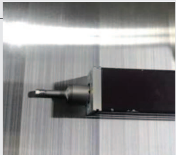
Measure the surface after grinding operation
