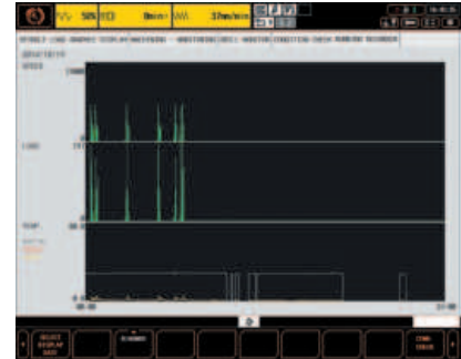
▲ Running recorder Operation status of milling spindle (rpm / motor load) can be recorded for up to one year.
