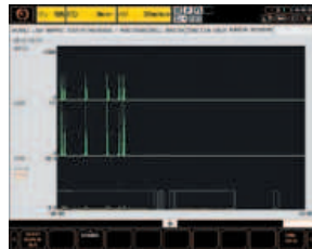
▲ Running recorder Operation status of milling spindle (rpm/motor load) can be recorded for up to one year.
