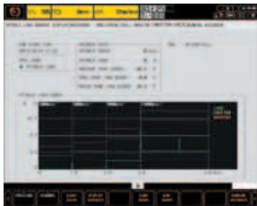
▲ Condition Check Temperature as well as the motor load can be displayed.
