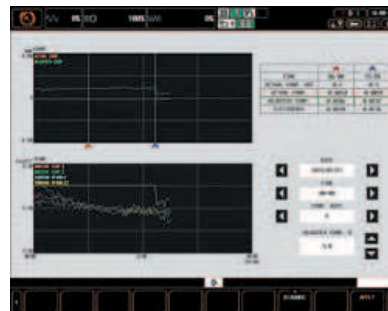
Temperature and compensation is displayed on screen. The operator can adjust compensation by looking at the data.
